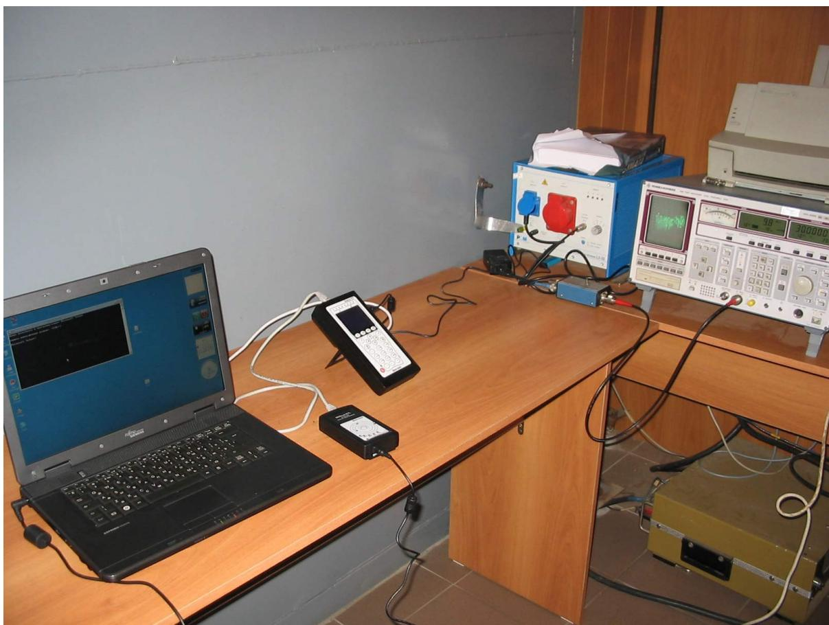
**Telecommunication Ports Conducted Emissions Test Configuration**
